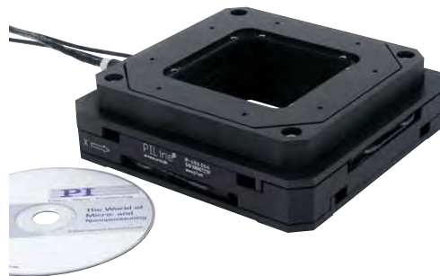
M-686 open-frame stage with P-541.2DD piezo scanner on top, providing a resolution of 0.1 nm and a scanning range of 30 x 30 \mu\text{m} . The system height of the combination with the P-541 XY (or Z) piezo scanner is only 48 mm
