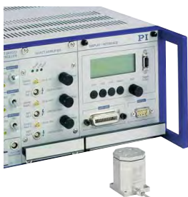
E-536 controller with P-363 PicoCube® pico-positioning system
